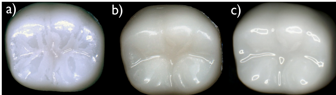
Figure 2: Monolithic full anatomic Y-TZP InCoris TZI crowns, a) Super Speed, b) Speed, c) Long-term sintered
