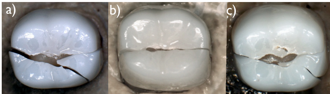
Figure 4: Y-TZP bulk fracture after single load to failure test after mouth-motion fatigue; a) Super Speed, b) Speed, c) Long-term sintered.
